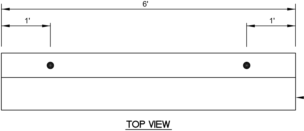
RECYCLED PLASTIC/COMPOSITE WHEEL STOP
