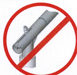
Slot in rafter allows water corrosion
