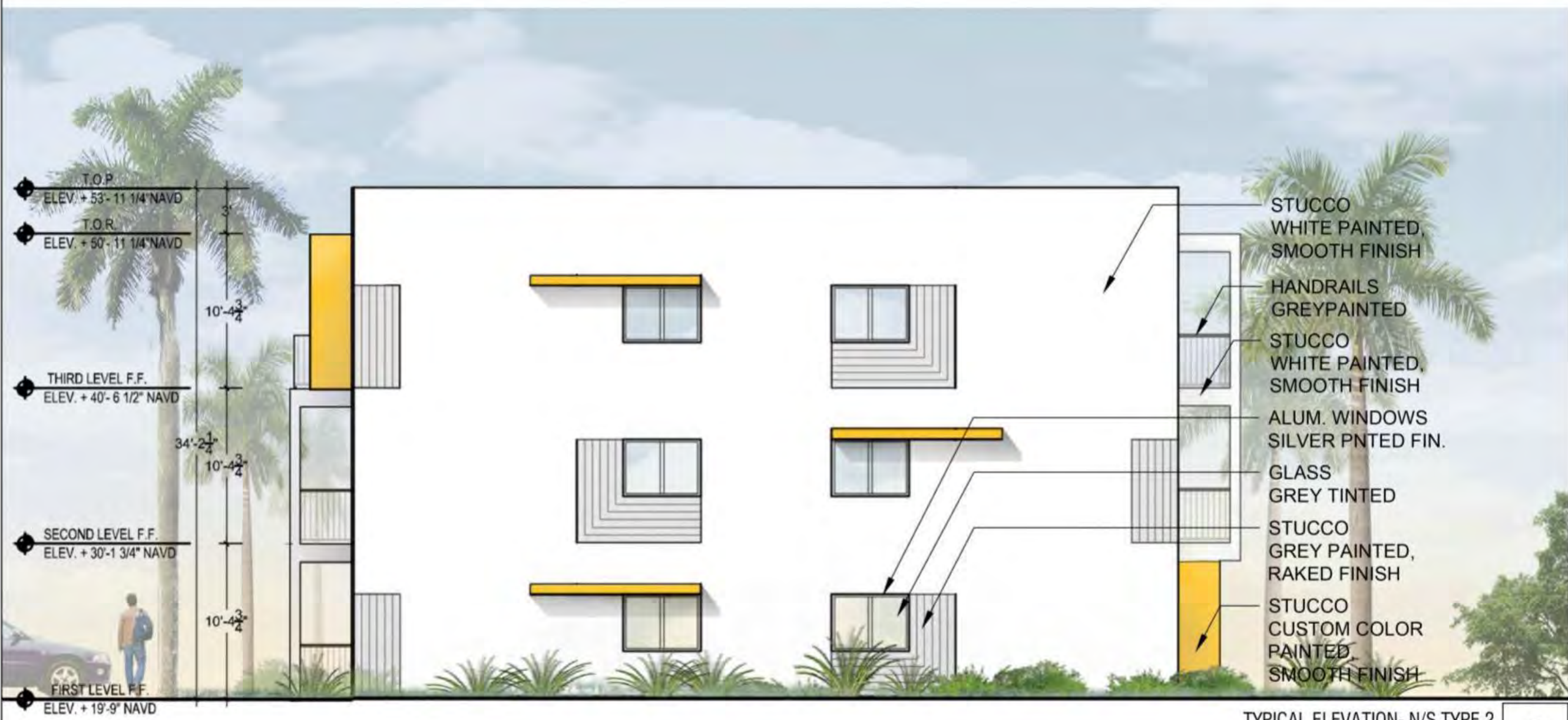
TYPICAL ELEVATION- N/S TYPE 2
