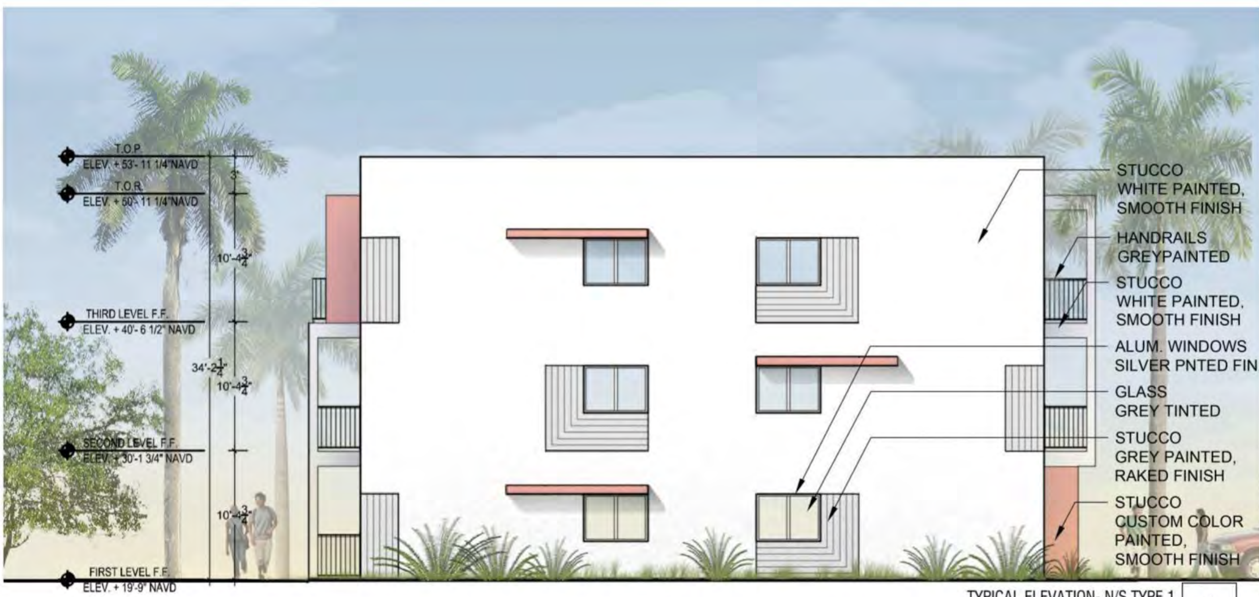
TYPICAL ELEVATION- N/S TYPE 1
