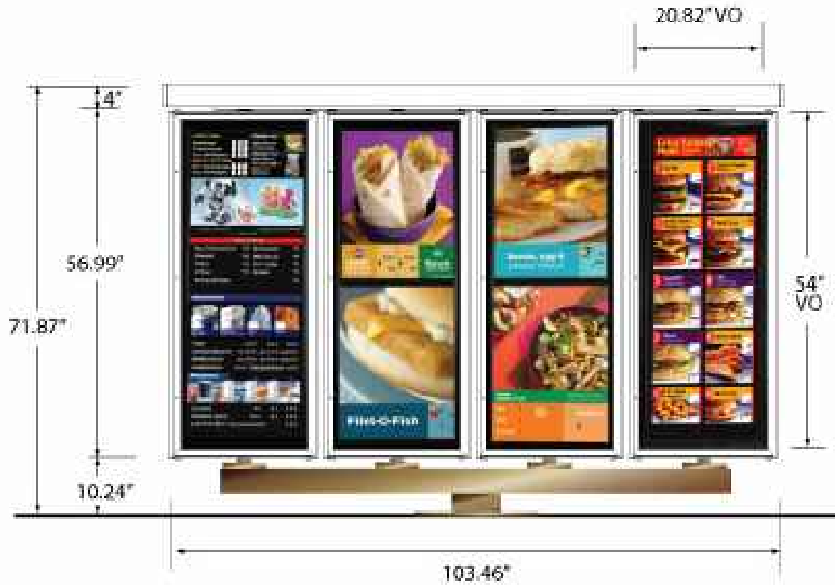
B OPO OUTDOOR MENU BOARD 4-COLUMN SIGN AREA CALCULATION: TOTAL SQ. FT. = 1.735' * 4.5' * 4 = 31.23 SQ. FT. EACH
